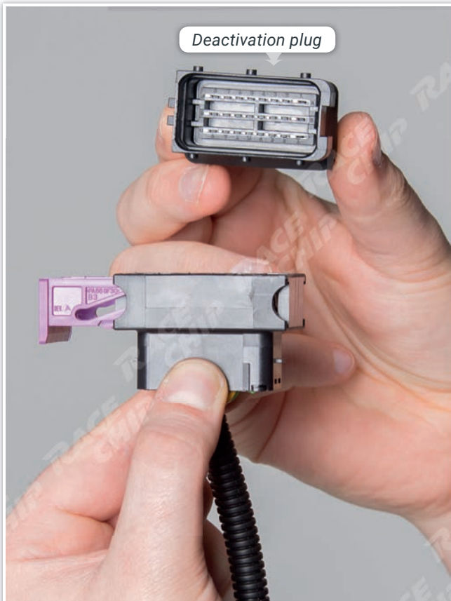
Wiring harness with deactivation plug removed
